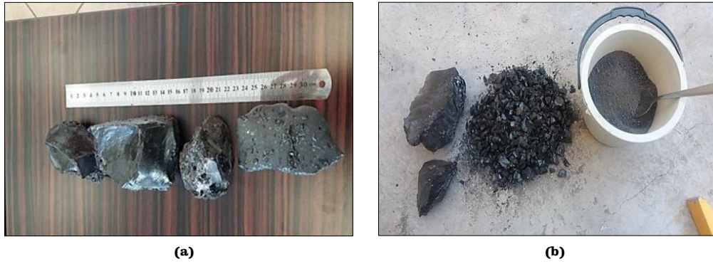
Fig. 1: The used steel slag in the laboratory tests, A-Large particle size, and B-crushed and powdered. (Source: Researcher)
